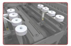
ENTRY TOP COMPRESSION UNIT Assists with proper sealing of top HSC flaps.
