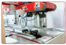
**HIGH SPEED TOP & BOTTOM BELT DRIVE SYSTEM** Providing you the stability and speed for high speed applications.
