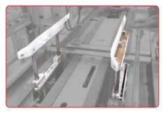
**INNOVATIVE LIFTING STATION** Ensure proper separate sealing of the lid and bottom of HSC cartons.
