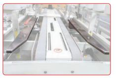
LID LIFTING GUIDE RAILS Maintain HSC height for separation of HSC box lids.
