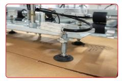
**VENTURI SUCTION CUP SYSTEM** Ensures reliable attachment by amplifying air pressure for strong grip on cartons.
