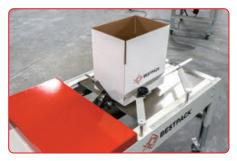
ADJUSTABLE RAIL WIDTH MECHANISM Manually Adjust the rail to provide support for a wide range of cartons.
