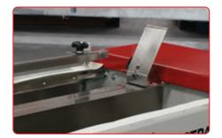
**AIR MICRO SWITCH** Switch activates to close the bottom flaps and holds the carton in a tilted position.
