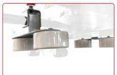
TOP COMPRESSION ROLLERS Eliminates the carton's top gap for added product security.
