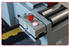
**EMERGENCY STOP & START BUTTON**Instantly shuts off power during emergencies, offers easy access for operator to restart machine.
