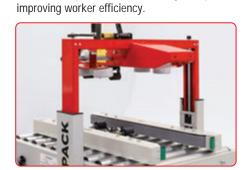
**DUAL TELESCOPING MAST**Stronger design, capable of precise adjustments resulting in a clean, consistent seal.
